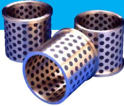
LUBRON® HP self-lubricating bearings feature a proprietary PTFE-filled solid lubricant embedded in a cast bronze backing. Specifically designed for hydropower turbine wicket gate applications, LUBRON HP bearings require no maintenance and provide superior performance throughout long service life.
